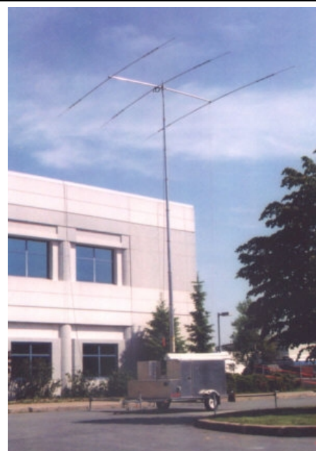
The EMO repeater trailer deployed for Field Day 2003 at the EOC
