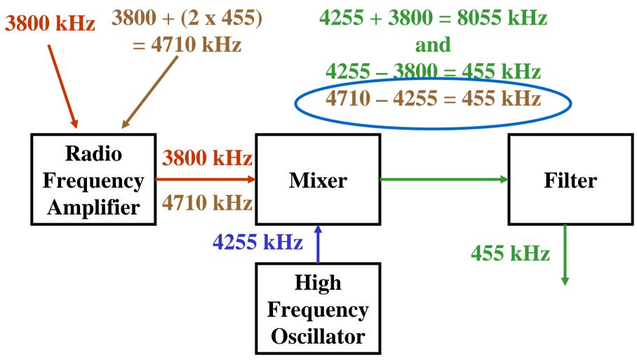
3800 kHz + 455 kHz = 4255 kHz
