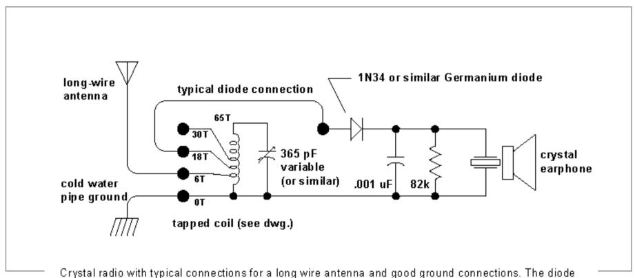
Crystal radio with typical connections for a long wire antenna and good ground connections. The diode is connected for weak signals and moderate selectivity.
