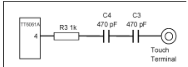
Figure 1: Unmodified touch terminal circuit - simplified diagram.
