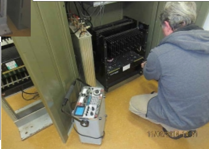
Site visit results: Found DC power supply for port 3 radio was dead. Replaced with original DC supply (fixed by Lorne) Removed TX channel element and cleaned up IDC pot Re-adjusted IDC to spec and rechecked TX deviation on Port 1. Next visit Port 3 radio will be programmed for active high COS along with RLC controller. 73, Lorne & Brad
