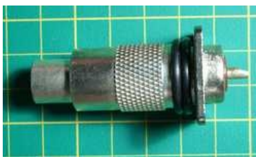
Place the O-ring(s) at the base of the SO-239 barrel and use the PL-259 coupling ring to compress them into a weather-tight seal.
